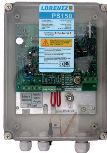
PS150-Centric C-SJ5-8 Controller, Pump and brushless motor
